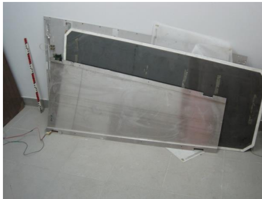
One bottom gap and the top cover equipped with 3 FEBs.
