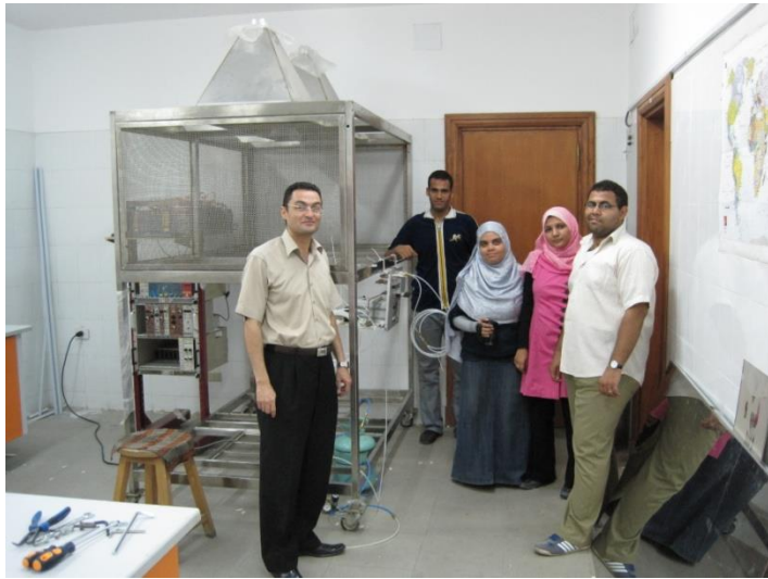
The team standing next to the cosmic stand with temporarily mounted gas mixture crate and 3 NIM crates and CAEN HV/LV crate installed in the shortened CERN rack.
