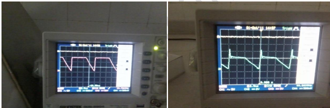
Figure.7two amplified signals from the two outputs of the simple detector (there seems to be a problem with one of the outputs)
