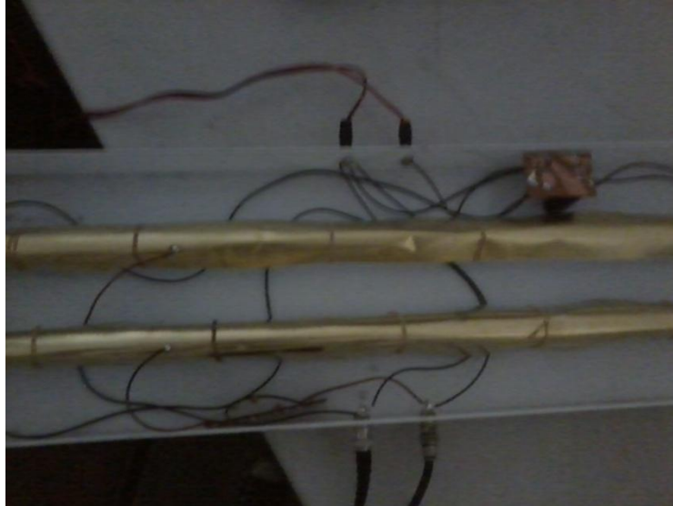
Figure .6the fluorescent detector using larger fluorescent tubes
