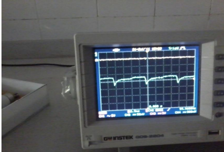
Figure.9 coincidence signal between the two output of the simple detector
