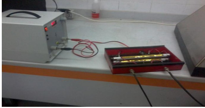
Figure.1 the simple detector constructed at Helwan Ps. Since we're using two tubes we've two out puts
