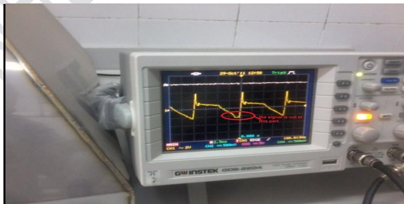
Figure.3 the amplified signal coming from the simple detector (there's no negative peak and also as the red mark refers there's a cut in this signal)
