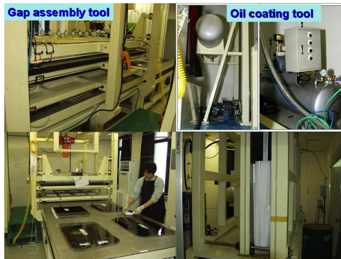
Figure 2. Gap bonding facility (left column) and linseed oil treatment facility (right column).
