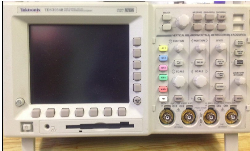
1 Digital Phosphor Oscilloscope, Four channel color, Ktronix TDS 3054B, 500MHz. 5GS/s.
