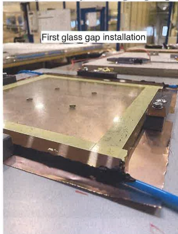
Figure 44: Final stage of chamber assembly.
