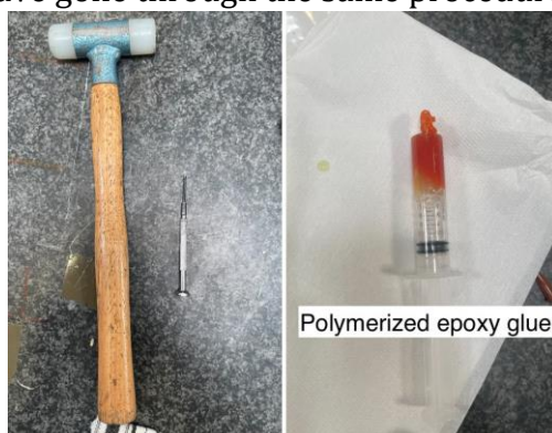
Figure 26: Tools used to remove the glued glass gap.
