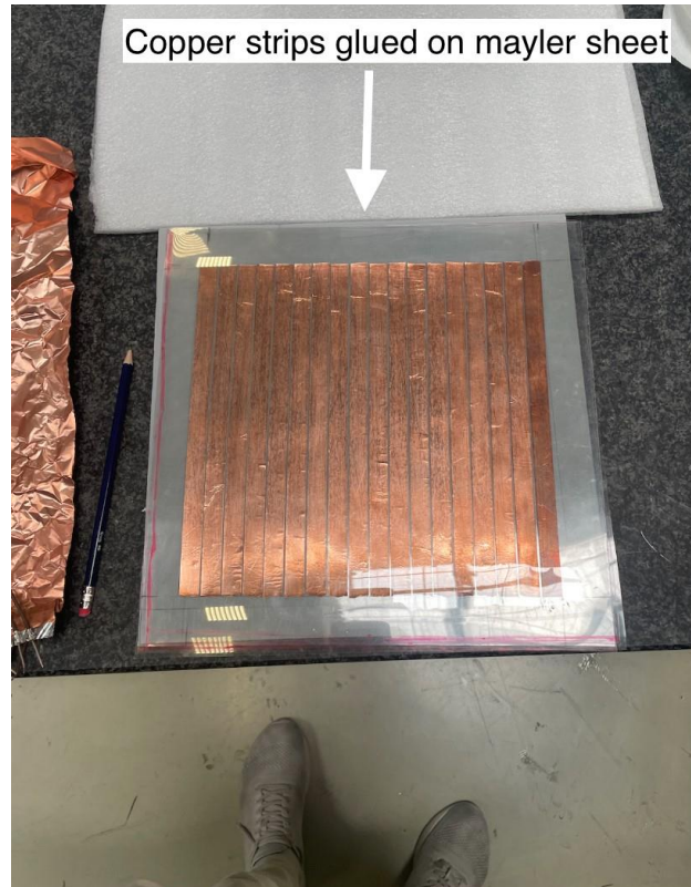
Figure 46: Myler sheet with 20mm copper strips.
