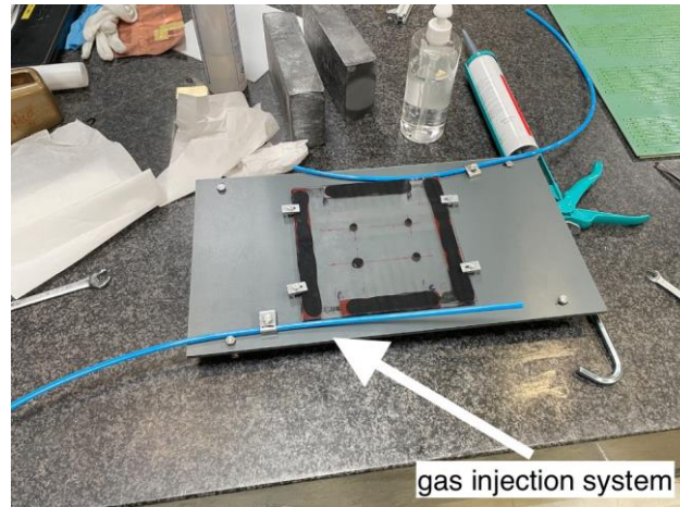
Figure 33: The Polycarbonate gap connected to the PVC platform with the polymer tube by using clamps and screws.
