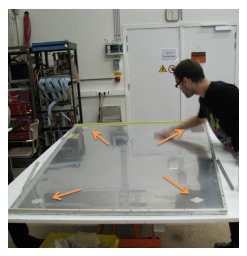
\*Carefully position the doublesided tape on the hcp bottom panel before removing the cover paper of the tape, then let the mylar roll onto the pieces of bared tape to avoid creases.
