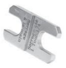
The shim shown above (5/16 CCS 8) is to verify that the 5 elements have been put in the correct orientation ready for assembly. The 5 elements are the pipe(8mm dia) the 2 ferrules, the union and the nut.
