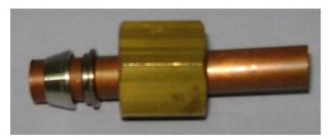
The pipe diameter I assumed was 8mm. I was not able, with finger force, to put the olives/ferrules into the nut shown and so no coupling was made. This is not surprising as the nut is an old fashioned Legris and the SS ferrules are perhaps Sagana/Rotarex. The correct components MUST be used.
