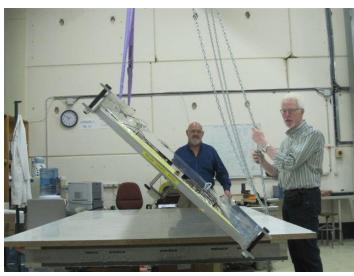
Bolts foreseen to pick up the frame in every position Forseen wheels at the end of each U profile From horizontal to vertical position
