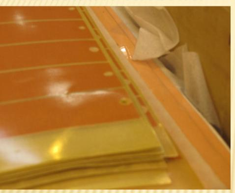
The strip's ends have no soldering points made by a special heat locating zones as they are in the previous productions like RE1,RE2 and RE3. Due to this it is not possible to localize the soldering temperature in one point and make the soldering with minimum heat. We have a situation that ALL the Cu Strips were over burned and their contact end has no more glue contact with the fiberglass base of the readout PCB.
