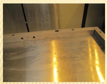
We have expected several boxes from each type. We found that inside lots of aluminum particles are left from the machining. Also they have very sharp edges which require shaping before use.
