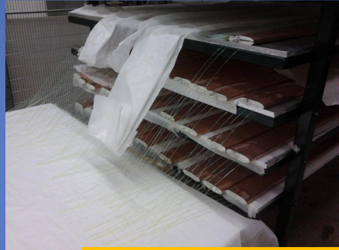
Scintillators with glued fibers
