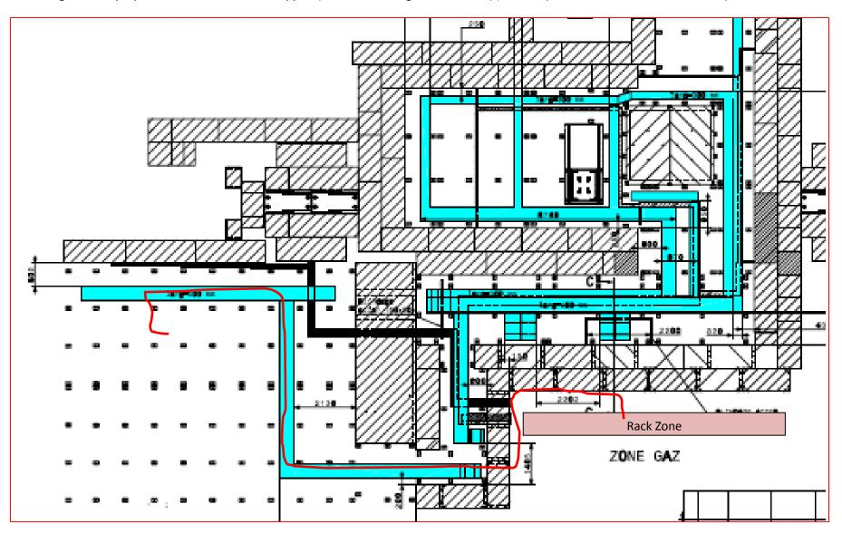
Cable length to the preparation area L = 35m Approx(includes 3m height at each end) ) In reality we measured 32m but without position definition
