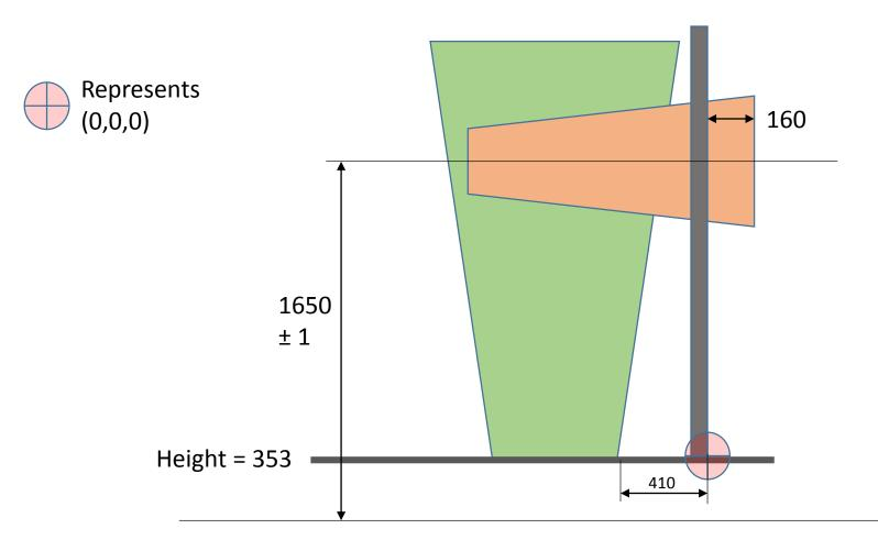
Nota. The horizontal chambers can roll in "x" so must be specified for each new position.
