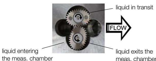
This technology allows precise flow measurement and dispensing of most clean liquids regardless of their conductivity, with other liquid characteristics having no or minimal effect on meter performance. This metering technology does not require flow profile conditioning or straightline runs as required with alternative flow technologies making the installation relatively compact and low cost.
