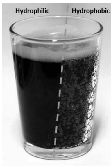
Fig. 10.24 The effect on beer foam and bubble formation at the beer/glass interface in a glass exhibiting both hydrophilic and hydrophobic surfaces. From ref (48).
