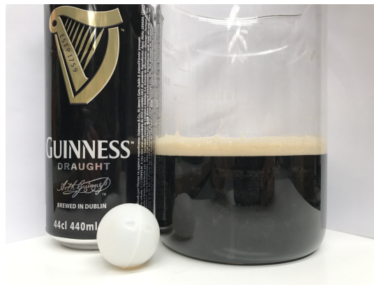
Figure 3. Widget inside a Guinness can. The hollow ball is filled up with pressurized gas at the same pressure than the can. When the can is opened, the widget breaks and generates a turbulent gas jet that introduces the mixing necessary to trigger foam formation.
