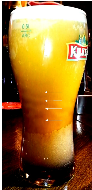
Figure 2. Waves in a freshly served pint of a stout beer. The arrows mark the location of the peaks in bubble concentration. The downward motion of the waves can be observed in the associated Video S3 (see Supplemental Materials). Note also the chaotic oscillation of the front that separates the recirculation bubble trapped by the thickening of the glass near the bottom and the downwards flow of foam near the wall.
