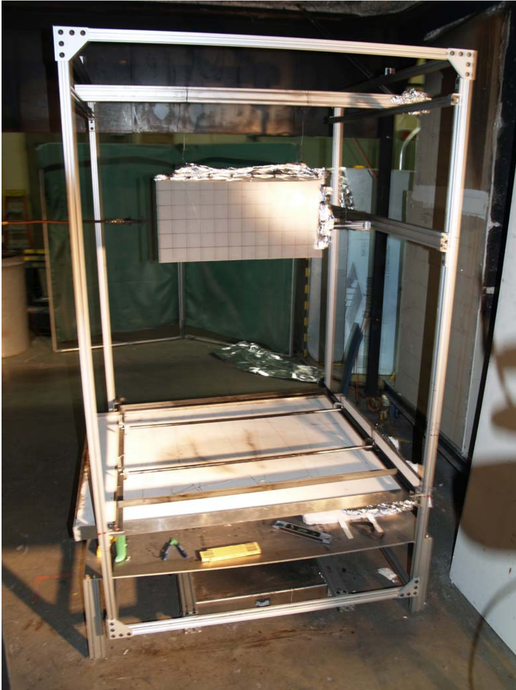
Figure 2. Overall view of the apparatus used for three-dimensional, melt pool fire-assisted fire growth tests. A thin sheet of polypropylene is shown in its high position above the Marinite catch surface (white sheet).
