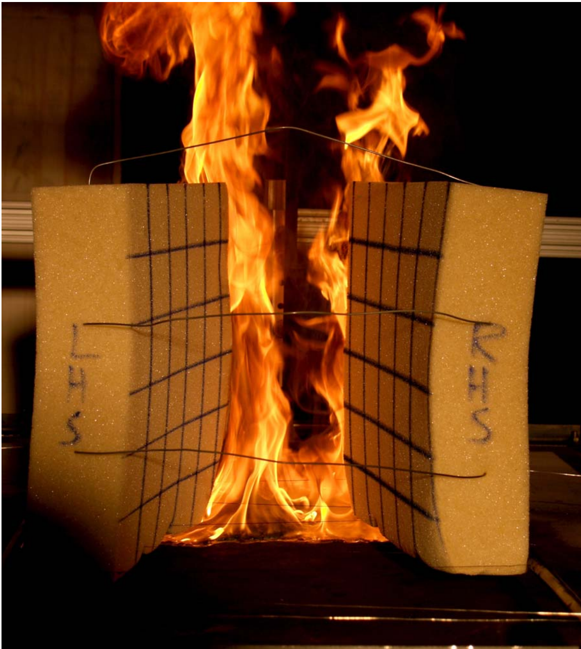
Figure 32. Vee test of L viscoelastic polyurethane foam, showing strong contribution from melt pool fire. Compare Fig. 31. Note differing shapes of flame fronts on interior surfaces of foam slabs.
