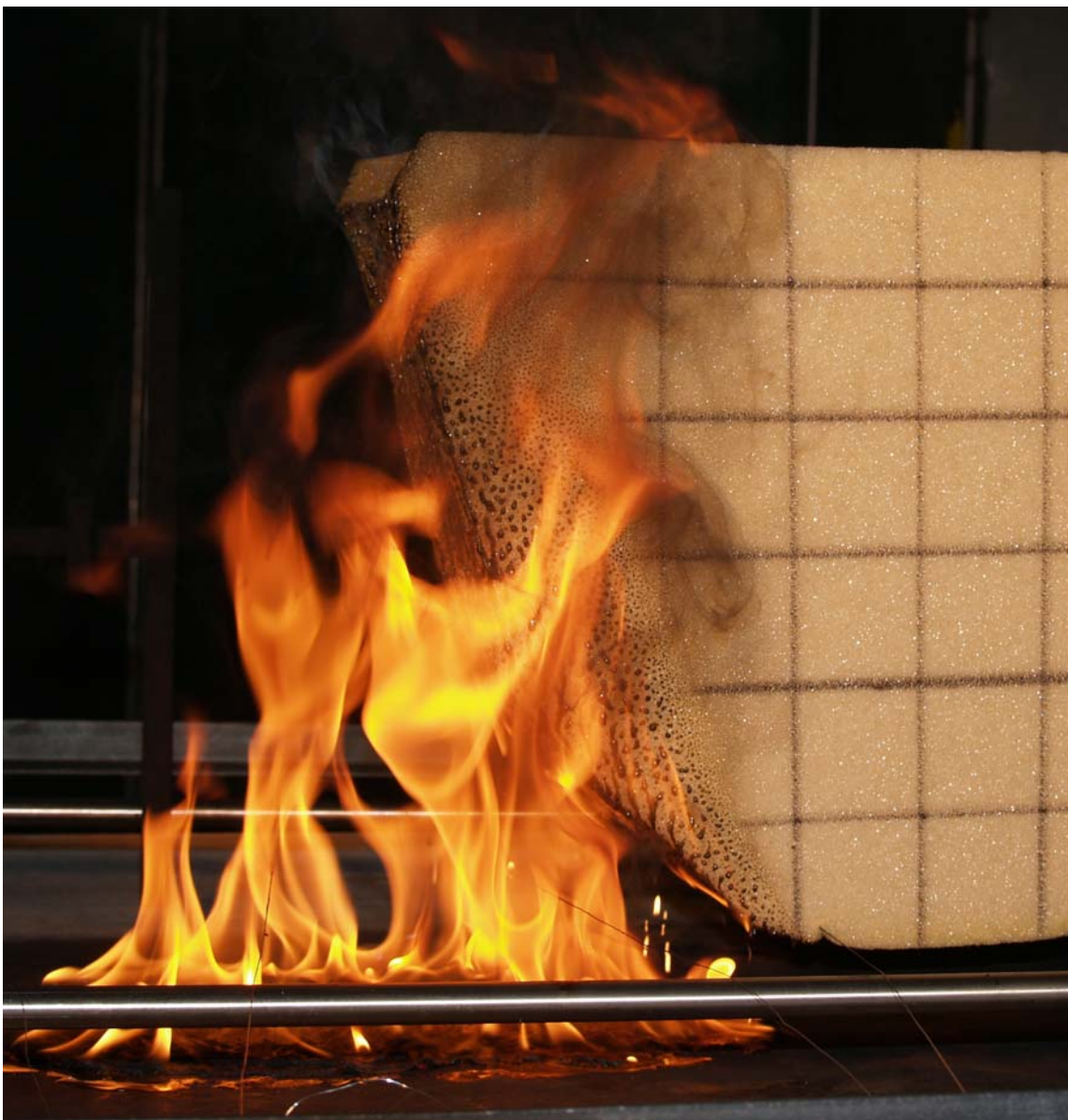
Figure 30. Side view of single vertical slab of L foam, burning from left to right, showing dominance of pool fire for this viscoelastic foam.
