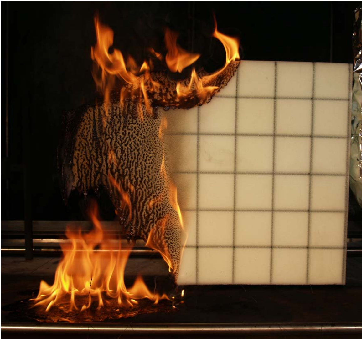
Figure 29. Side view of single vertical slab of flame-retarded Z'' foam burning from left to right. Note preferred spread on top surface where flow wake can create longer residence time for reactions.
