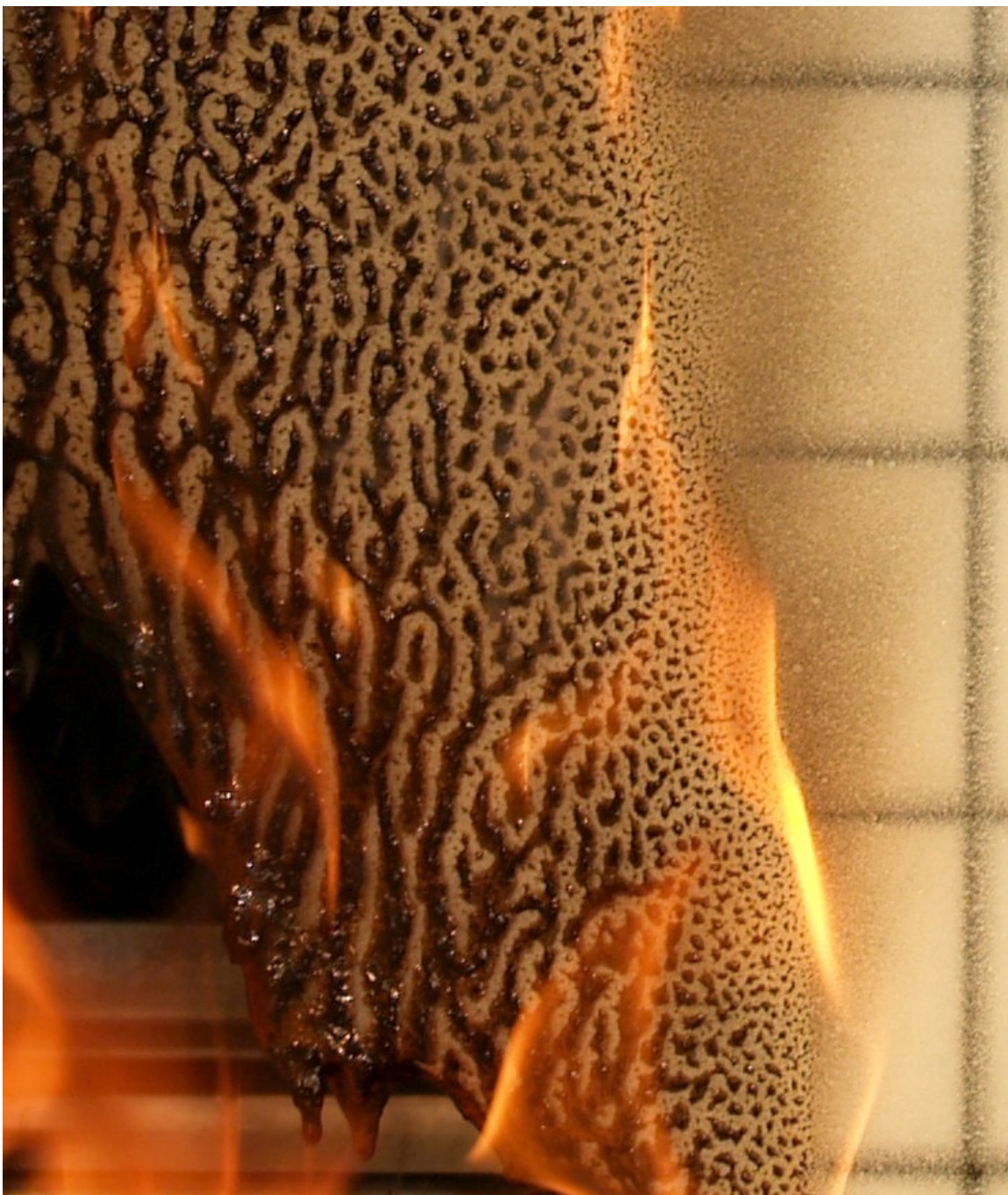
Figure 28. Close-up of burning zone on side of polyurethane foam slab showing melt bead coalescence and flow; Z'' foam. Flame zone is moving from left to right in photo. See Fig. 29 for overall view.
