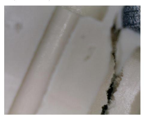
Brittle fracture is evident with low strength.
