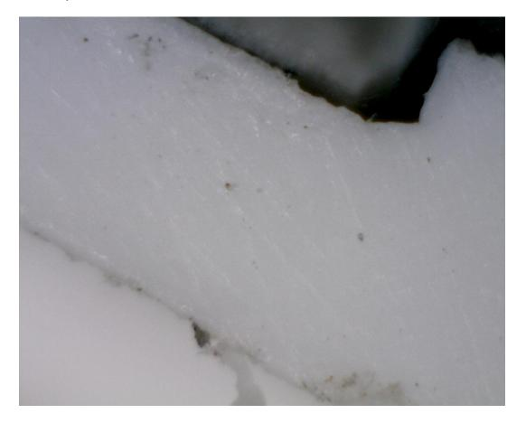
It would appear that the new version has been heat treated in a manner to form excess crystal growth, in an attempt to make the material more fluid for better mould filling as opposed to the older versions that remain more amorphous. The higher crystalline content may decrease electrical conductivity while reducing breakdown voltage.
