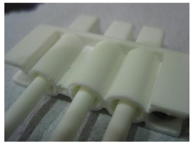
Different views, end on, showing that the intentional cavities between the pins has on the old version has now been removed and put into the "rear" of the connector where the potting will occur.
