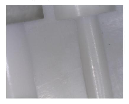
However of the 3 connectors opened, there are visible voids of smaller size than before.
