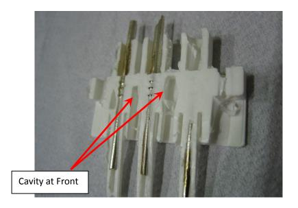
This then leaves rather small apertures (see below) for the potting liquid to enter and the air to escape. If the air cannot escape cavities will remain. This is in the area, as before, of the barbs on the pins, see later comments. In the new version the possible cavities will be more controlled in size.
