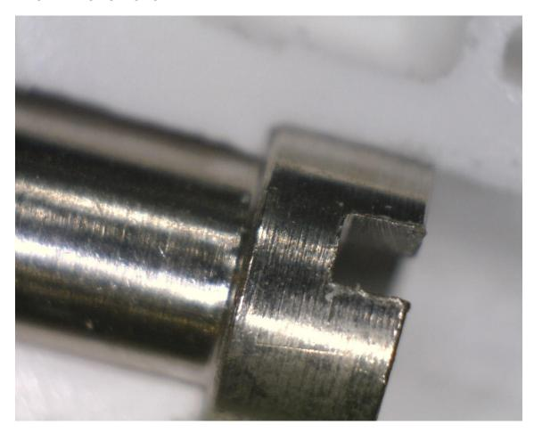
The screw thread is, in comparison, rather rounded off and is not so close to the sharp pin barbs.
