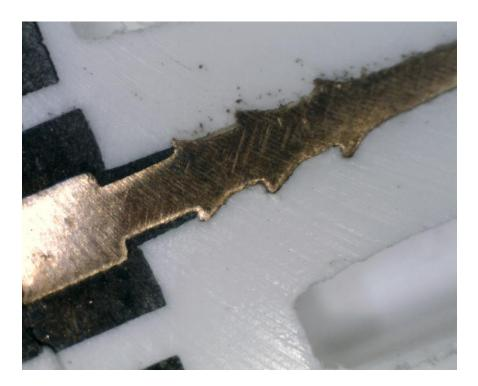
These are in proximity to the voids and the securing pins. The pin itself is not sharp edged BUT the screwdriver slot is not deburred AND has been damaged by the tool (too small?) used to tighten the pin.
