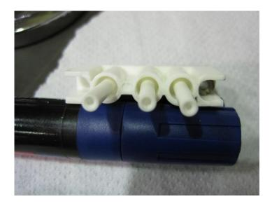
The connector cut open shows the entry of the cavities between the pins has moved to the rear of the connector.
