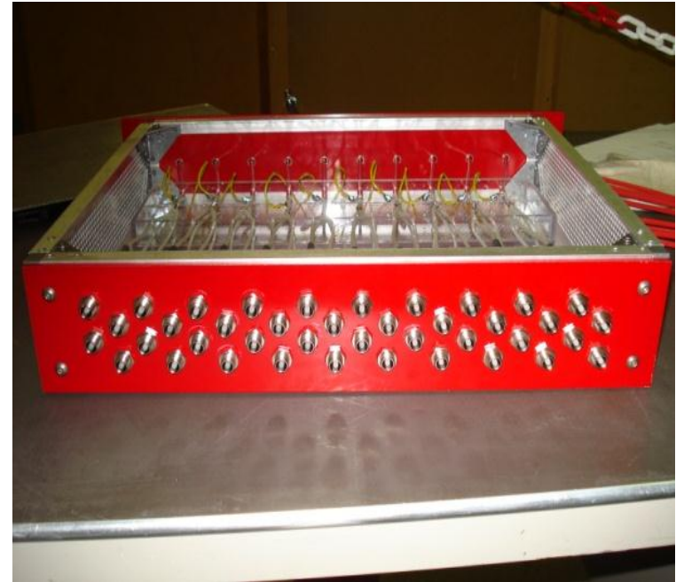
Output Side of Distribution Box
