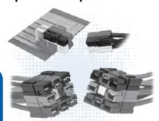
PP15-45 series are the smallest Powerpole® housings. They can be used for wire-to-wire or wire-to-board applications. Wire sizes from #20 AWG (0.5 mm²) to #10 (6 mm²) offer power capabilities up to 55 amps per pole. Finger proof housings and the ability to incorporate first-mate last-break ground connectors enhance the capabilities of this Powerpole® series.
