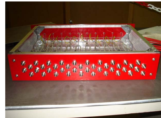
Output Side of Distribution Box
