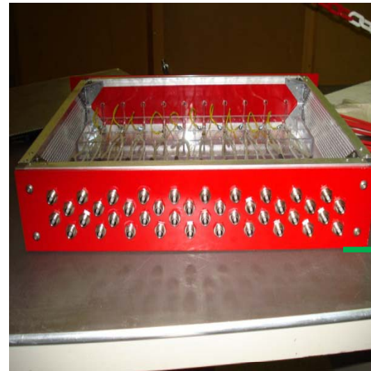
Distribution Box Output Side
