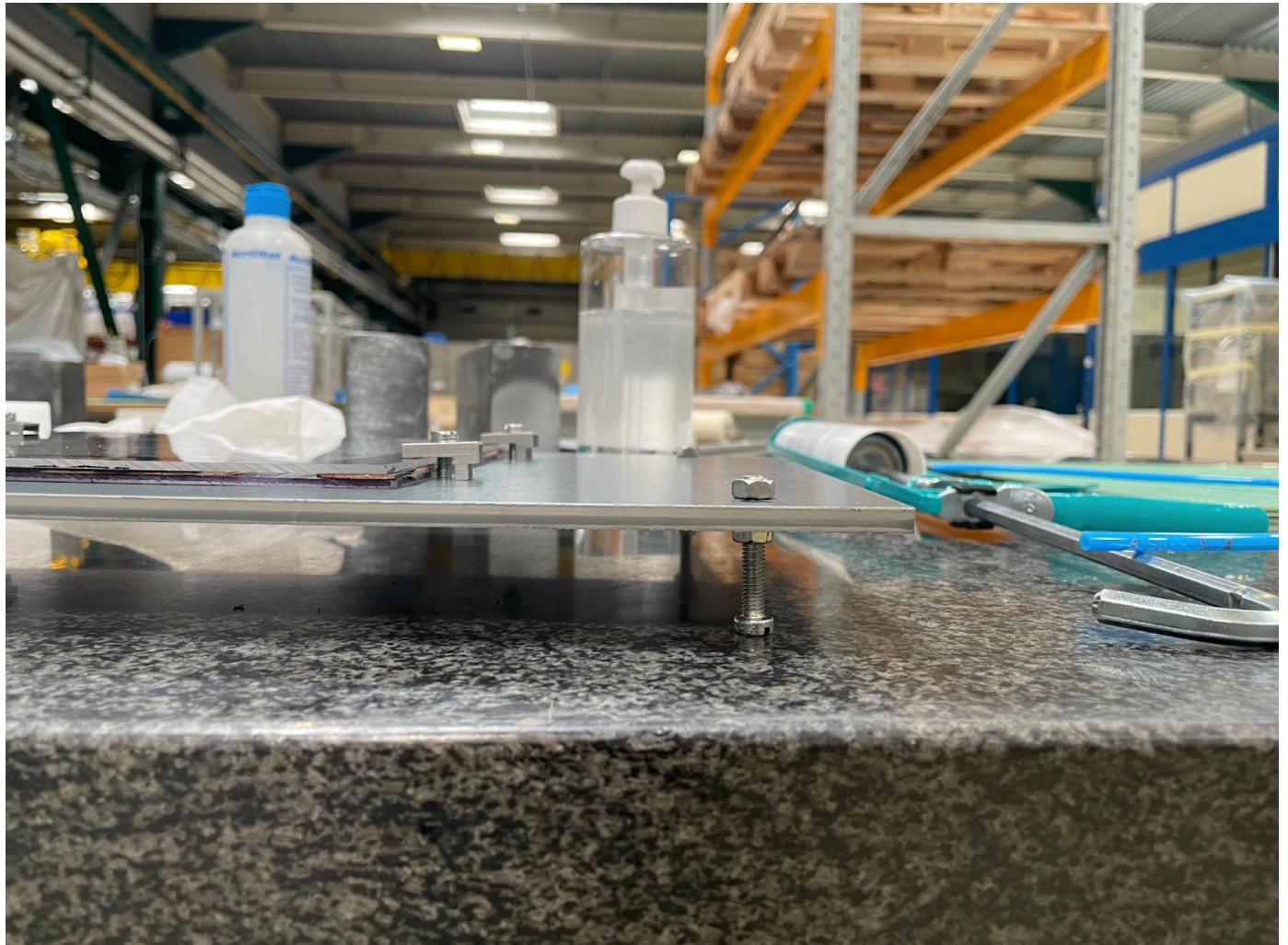
Figure 4.4: The legs for the PVC plate form that is made of one screw and two (...).
