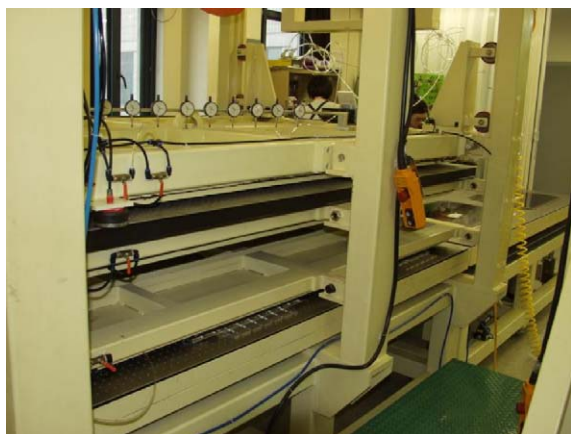
Fig. 7. Facility for the assembly of gas gaps. The facility equipped with three sets of flat metric tables and rubber chambers enables three consecutive assembly procedures.
