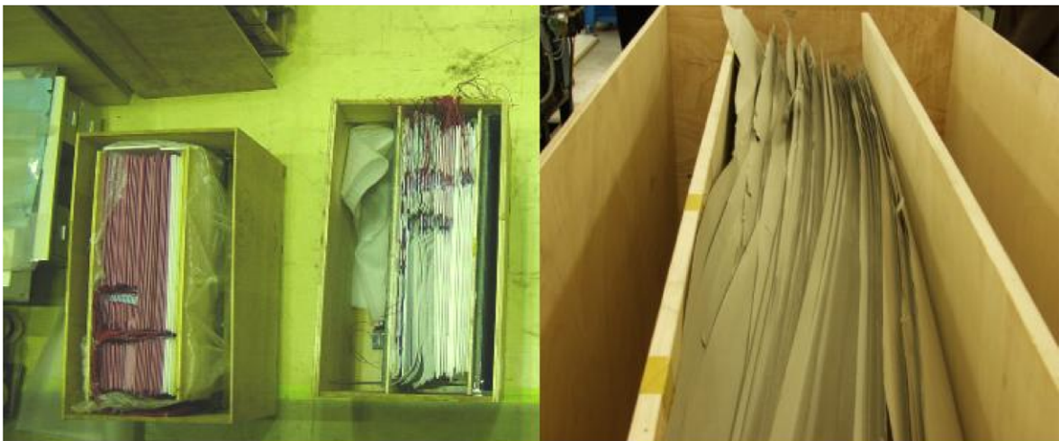
Fig. 12. Wooden boxes, equipped with four pre-loaded bars, specially designed for safe transportation of the gas gaps. The boxes are also used to ship the qualified bakelite sheets from Italy to Korea via CERN.
