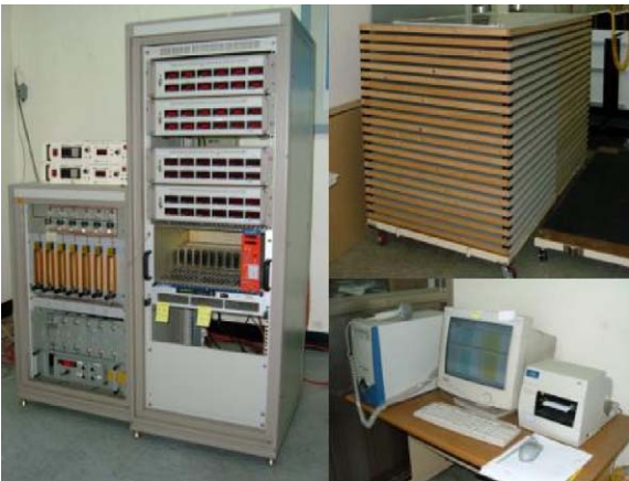
Fig. 9. Facilities for the high-voltage test. As shown in the left part of the figure, three high voltage supplies, four 12-channel current measurement devices, and a 6-channel gas supply system are used for the high-voltage test. The right part of the figure shows 22 RE2/2 full gas gaps, placed on multi-layer shelves, for the test. After completing the high-voltage test, a bar code is assigned to each gas gap for later tracking.
