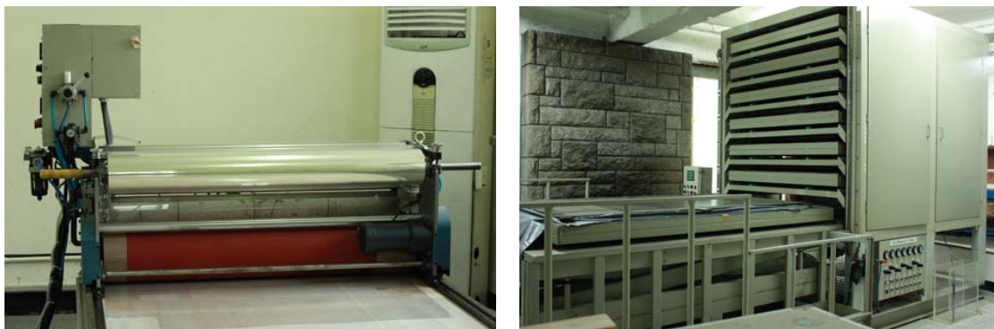
Fig. 5.1: a) electrode insulation machine; b) gap assembly machine.
