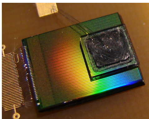
Figure 9.15: Bump bonded detector.
